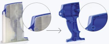
An end-use power tool handle before and after soluble support removal
